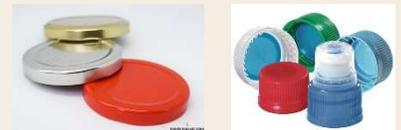
**Plastic caps** are usually made of a different type of plastic than bottles. However, in recent years, plastic recyclers have developed a sink-float process where the PET plastic bottles sink, and the PP plastic caps float! This way the individual plastic types can be harvested.
